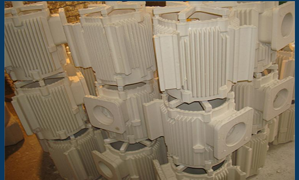
Model with Coating Applied
