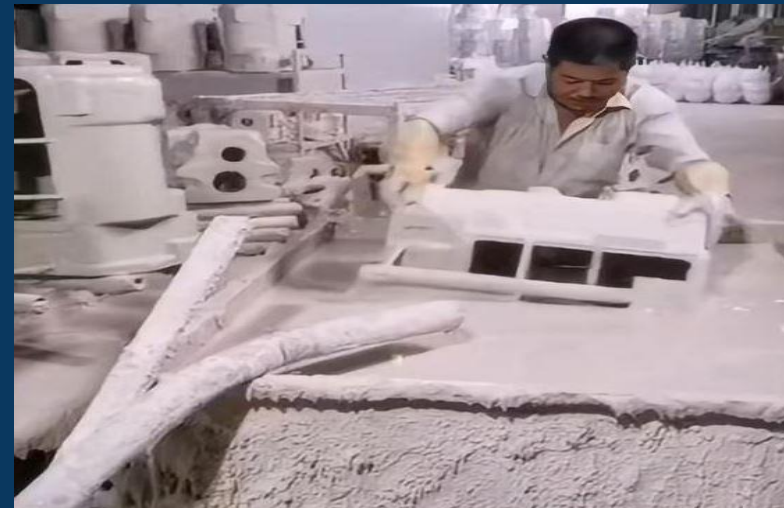
Lost Foam Water-Based Refractory Coating Dipping Site
