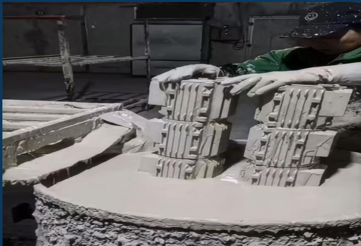
Lost Foam Water-Based Refractory Coating Dipping Site
