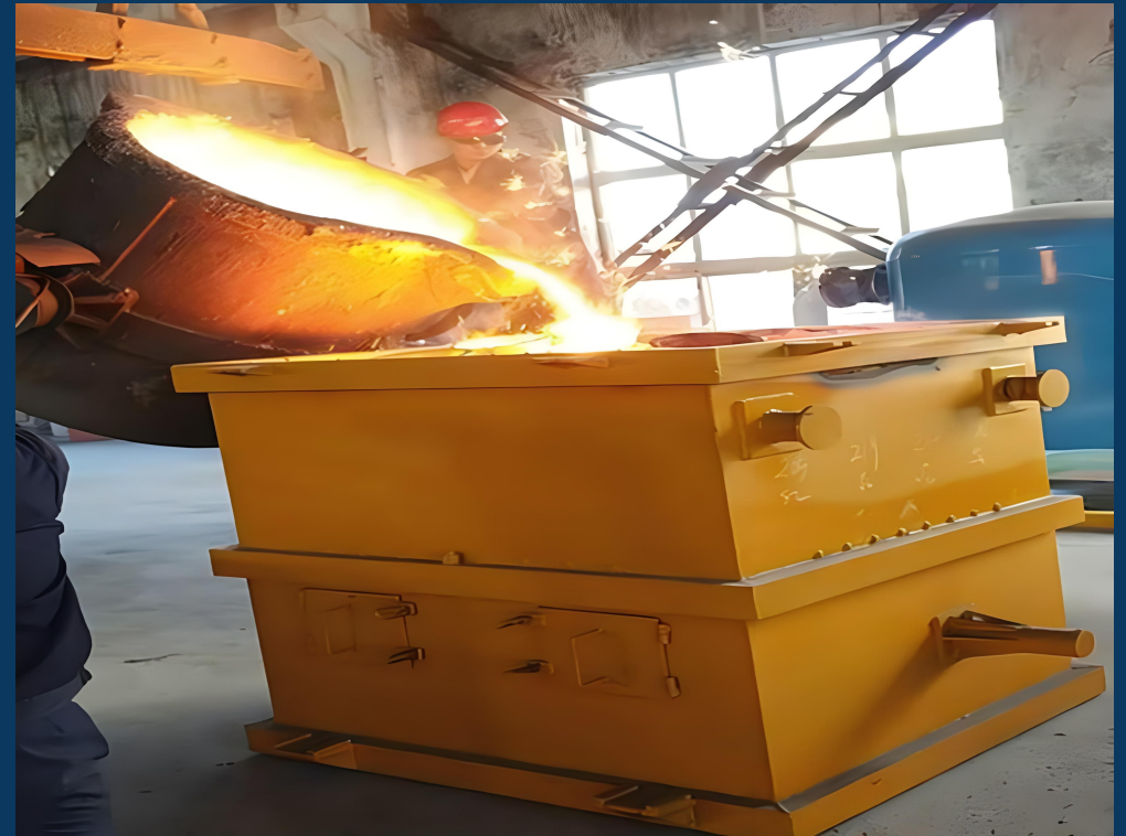
On-site Molten Iron Casting
